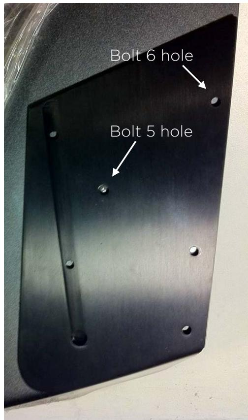
The ¼” hole through the deck lid bottom skin should be drilled from the bottom side using the drill guide in the image below. Cut out the image, which prints to scale, and use it as a drill guide. The head of Bolt #5 (M6 x 1 x 60 MM long, McMaster number 92095A254) will sit on top of the mounting foot / plate. The nut sits on the bottom side of the trunk lid. The bolts can be secured using the included washers and nyloc nuts, or one of the stock nuts that held the stock wing in place.
