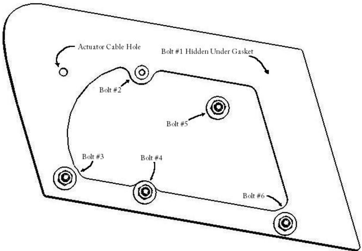
Top View of the passenger side gasket.
