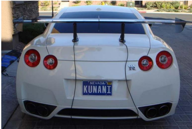
Once positioned, three holes should be drilled per upright. Two are clearance holes for the M6 studs, the third is for the power cable. The three holes are the same as the holes drilled in the carbon fiber feet.
