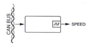
The CAN Adapter has built-in diagnostic LEDs to indicate CAN Bus status and speed pulse output to aid the installation process. After power-up:
