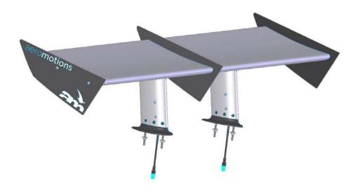
In order to use the stock GTR tune, the wing needs to be mounted in the correct position. The S2 wing mounts with four M6 studs that are permanently mounted to the bottoms of the Power Pods. These can be cut to length. The electrical cables that run to each power pod have a connector (shown in blue) that needs a clearance hole to pass into the trunk.
