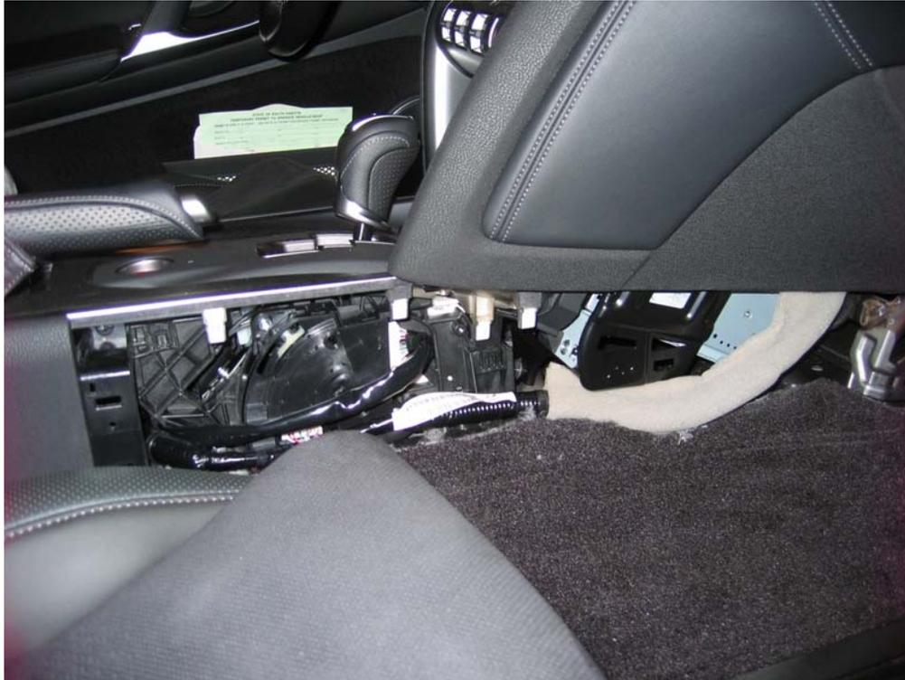
Behind the DVD head unit, there is a WHITE plug with 20+ positions. From the rear of the unit, it would be on the top left corner. From your passenger side view, it's the closest to you on top. Near the center of the TOP of the plug, is a red power line, right next to that is a VIOLET line. The violet line is the VSS wire. *Note, Australian, and British GT-R's have a light green VSS wire.*
