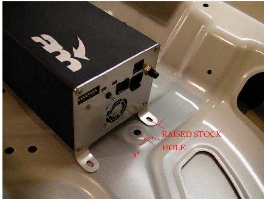
Pass the actuator cables through the existing holes in the trunk as shown in the picture above. The cables should pass through the existing larger holes in the top and bottom skin of the trunk. *Note, the short cable is for the left hand side.*
